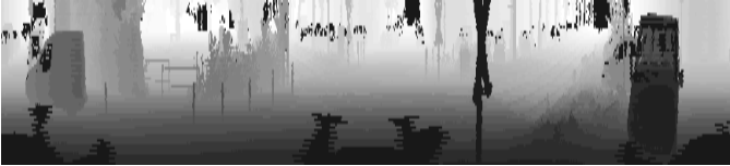
Fig. 4: LIDAR data representation as a spherical image. Row represent the elevation, Columns the azimuth and the value of each pixel represent the depth of the detection.
