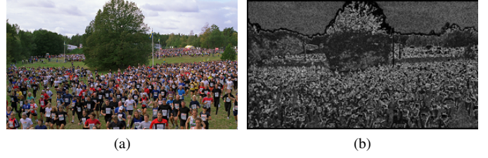
Fig. 2: (a) For crowdrun video sequence, Absolute difference (original-HVSP) for pre-processed frame(exaggerated by 100 times).
