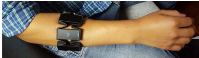
Fig. 3. Location of the Myo armband on the forearm.
