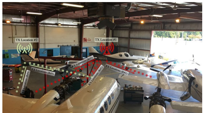
Fig. 3. Photograph of CUB maintenance hangar, showing several transmitter (Tx) locations and receiver (Rx) paths.
