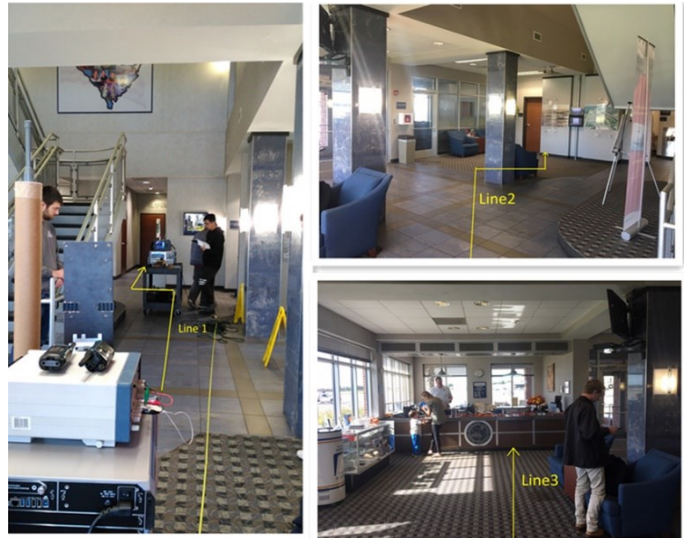
Fig. 2. Photographs of 1 st floor of CUB terminal building, showing LOS receiver (Rx) travel paths from transmitter (Tx) perspective.
