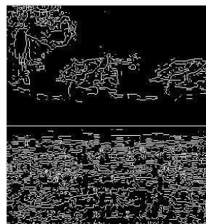
(j) JPEG H = 0.45 bpp PSNR = 32.23 dB SSIM = 0.97
