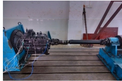
Fig. 3. The gearbox test rig
