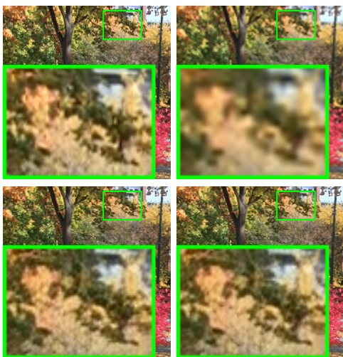
Fig. 5. Qualitative comparison between VSRResFeatGAN (2nd row, left) and S-VSRResFeatGAN (2nd row, right) on scale factor 3, with ground truth (1st row, left) as well as bicubic result (1st row, right). The enlarged region in our S-VSRResFeatGAN's output maintains clearer outline and is closer to the ground truth.
