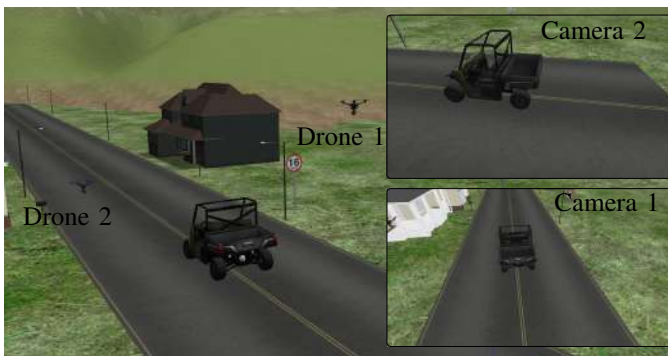
Fig. 5. Simulation with two drones. The target follows a straight line along the road. At that moment, Drone 1 and drone 2 are performing a CHASE and LATERAL shooting actions.
