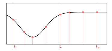
• Lipschitz filter is always stable  $\Rightarrow$  Either the eigenvalue doesn't move. Or the filter doesn't move
