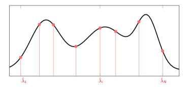
• Small deformations may result in large filter variations for large  $\lambda$  if filter is not integral Lipschitz
