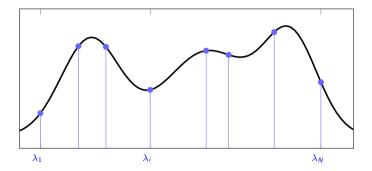
• Frequency response is the same no matter the graph  $\Rightarrow$  It's instantiated on its particular spectrum
