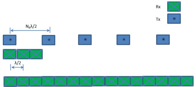
Fig. 1. Illustration of the MIMO system with  $N_T = 5$  transmitters and  $N_R = 3$  receivers. An equivalent array with receiver elements having the same aperture length of the MIMO system is also shown. We note that the system with receiver elements is fully sampled in the angle domain.
