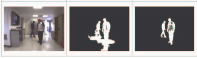
Fig. 3. The figure shows the results obtained by motion detection and shadow removing algorithms on images acquired in a laboratory. The first column shows the original image, the second column shows the segmented image obtained by only motion detection algorithm, the third column shows the image obtained by motion detection and shadow removing algorithms.
