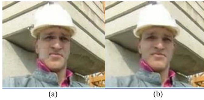
Figure 7. Frame 34 of QCIF FOREMAN sequence encoded at 40Kbps (a) Without filter (b) With loop filter
