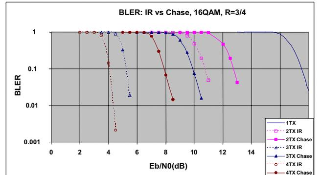
Fig. 8 HARQ type 2 residual BLER: IR vs. CC comparison.
