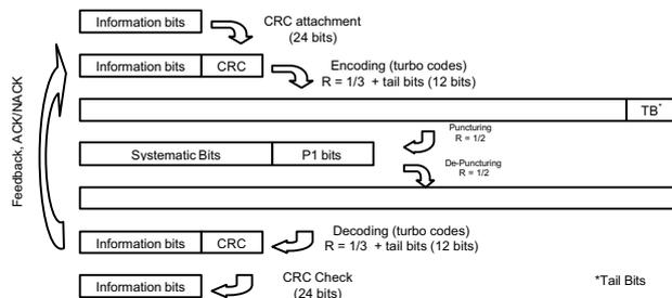
Fig. 2: Data flow graph for HARQ type 2 scheme. In the Incremental Redundancy case, the puncturing pattern changes at each retransmission.
