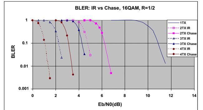
Fig. 7: HARQ type 2 residual BLER: IR vs. CC comparison.
