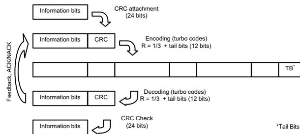
Fig. 1: Data flow graph for HARQ type 1 scheme
