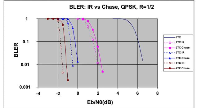
Fig. 6 HARQ type 2 residual BLER: IR vs. CC comparison.
