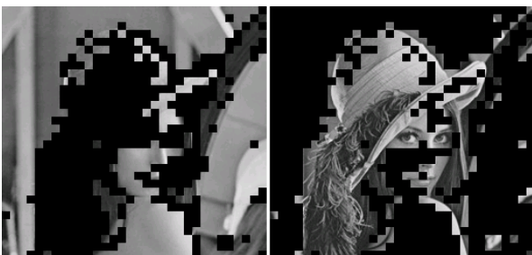
Figure 3: Areas with low (left) and high (right) EOBs in 'Lena'; others are masked out
